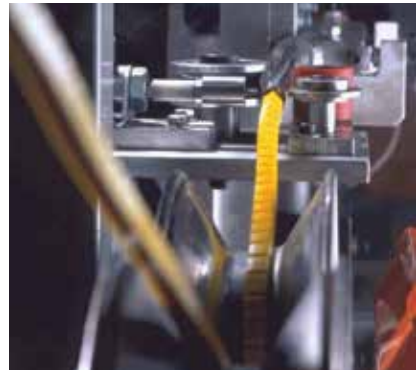
Notching machine and other downstream equipment for customizing extruded belting.
